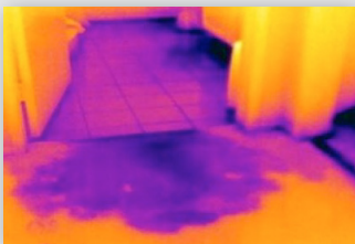
Localization of heating pipes and leaks
