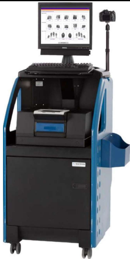
Figure 8: Ruggedized LiveScan with Adjustable Platen. Because the platen is adjustable in height, a person in a wheelchair can be fingerprinted more easily.
