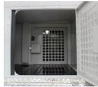
**Doors, Floor pans and the inside wall of the cages are made from .125 mill finish aluminum.**
