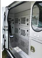
**Doors, Floor pans and the inside wall of the cages are made from .125 mill finish aluminum.**
