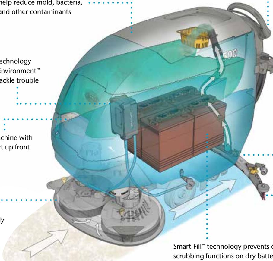
Smart-Fill™ technology prevents operators from using scrubbing functions on dry batteries and a control panel alert notifies operators when the distilled water tank is low
