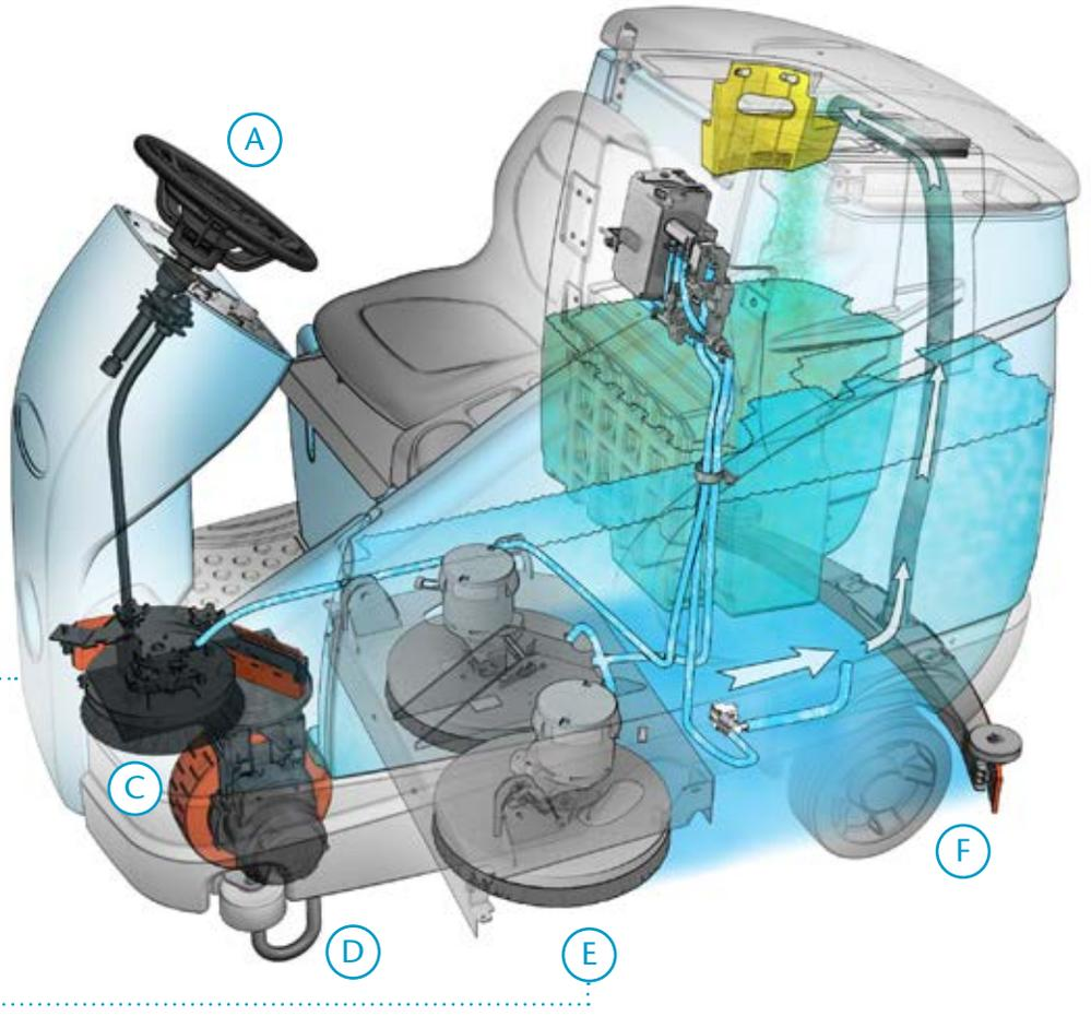
**A** Reduce operator fatigue and effort with controls placed in the center of the steering wheel for easy access.
