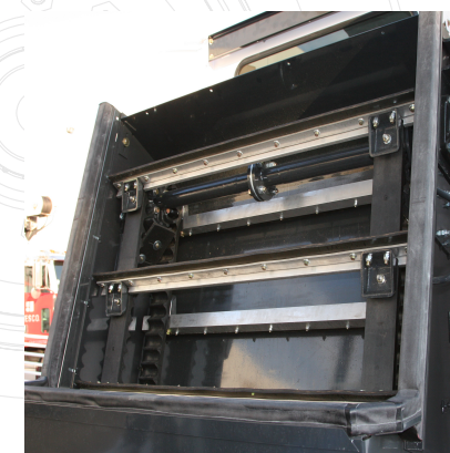
ABOVE Fuel System and Control Panel -Stainless Steel Tubes. -Stainless Steel Seal-lok Fittings. -Stainless steel devices w/O-ring fittings.
