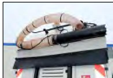
The robust rear-mounted suction system provides additional vacuum where you need it, such as emptying waste containers, shallow catch basins and loose debris.
