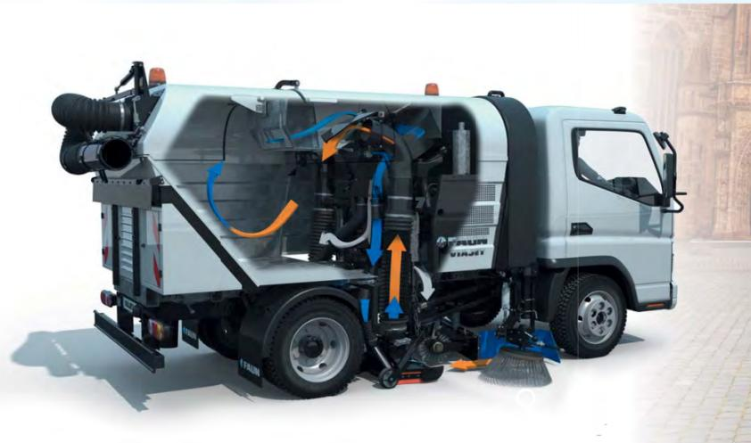
sweeper. Additional dust control is achieved by adding water to the recycled air. In winter the **Global V4** can operate at temperatures as low as 23 °F, due to the re-circulating air in the system being warmed to 59 °F, thus preventing the water in the suction tube and hopper from freezing.
