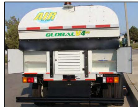
The **Global V4** offers two large storage boxes located at the rear of the sweeper
