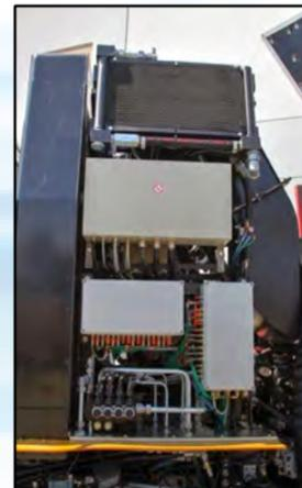
All valves and adjustments for the electrical, pneumatic, and hydraulic systems are located in one central console, which is maintenance -friendly and protects against water and dust.
