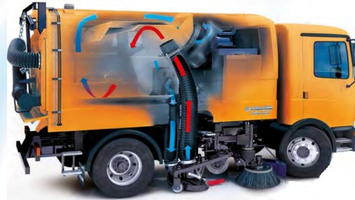
Minimal amount of dust is expelled into the working area at the rear and around the sweeper. Additional dust control is achieved by adding water to the recycled air. In winter the **Global V6** can operate at temperatures as low as 23 °F, due to the re-circulating air in the system being warmed to 59 °F, thus preventing the water in the suction tube and hopper from freezing.
