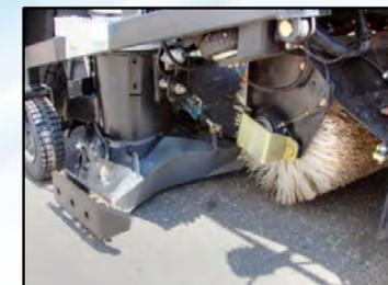
The channel brush or main transfer broom is mounted as a trailed brush and suspended separately from the suction nozzle. It is equipped with lateral shock absorbers and ground pressure adjustment in order to pick up heavy dirt off the road surface. **The pneumatically controlled adjustment of the main transfer broom offers the best possible performance in every working condition.**
