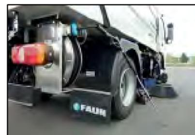
High Pressure Water Pump, along with hose reel and a lance allow for the ability to wash sidewalks, containers, etc...
