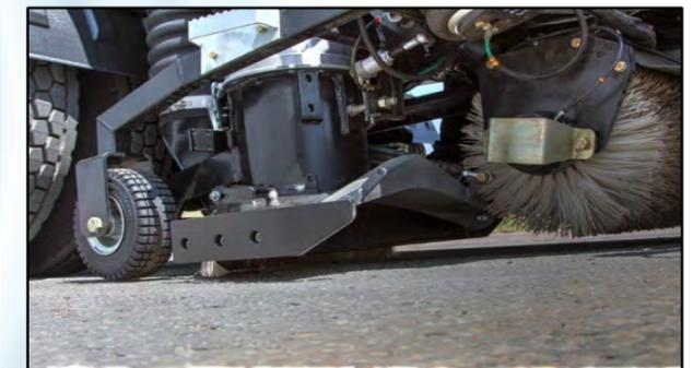
The **V-shaped Suction Nozzle** with its large aperture, made of 4 mm steel, conveys the swept material directly into the suction tube. This design enables the **Global V6** to lift the Heaviest of debris in any application.
