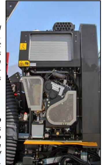
**Global V6 STANDARD** sweeping package includes **Tier 4 Final 2.0L 74hp Diesel engine** with a fuel consumption of **1.5 gallons per hour.**
