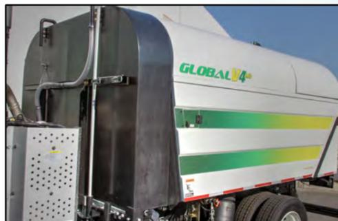
The fiber glass water tank is mounted in between fan and cab, providing additional noise protection as well as low Center of gravity. With Water Tank Capacity of 210 gallons you have plenty of water to get the job done!
