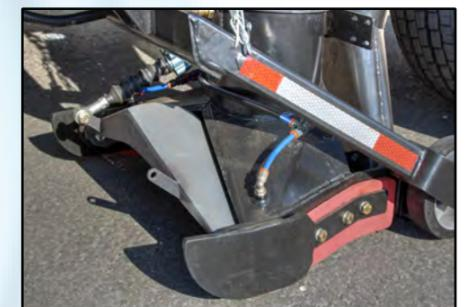
The **V-shaped Suction Nozzle** with its large aperture, made of 4 mm steel, conveys the swept material directly into the suction tube. This design enables the **Global V4** to lift the Heaviest of debris in any application.
