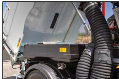
The twin water tanks provide a total tank capacity of 500 gal. of water. The primary fiber glass tank is fixed directly onto the sub frame under the hopper. The secondary tank, also made of fiber glass, is mounted in between fan and cab, providing additional noise protection. **SWEEP ALL DAY!**
