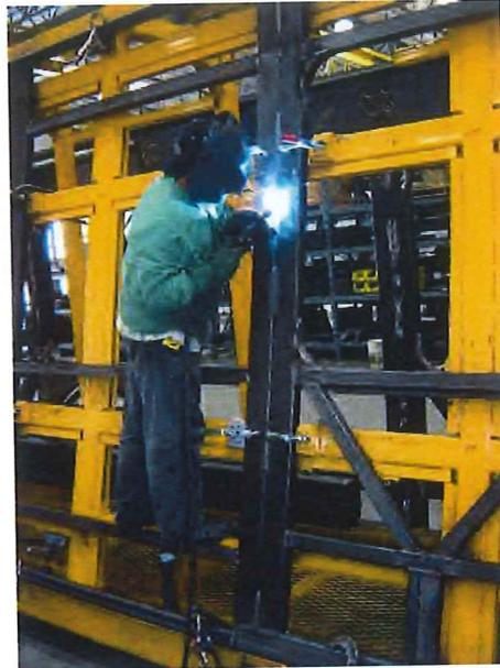
1. The inner walls of all tubular structures are coated with Ziebart - Formula A prior to tube cutting and welding. The entire cage is then fixture-welded for build consistency throughout the order.
