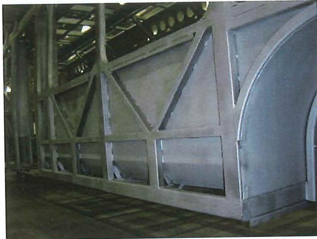
3. The frame assembly is moved into a grit-blast booth where it is blasted entirely with a 40/50 mix of steel grit medial. This process gives all steel parts a 1-mil physical profile for superior paint adhesion.
