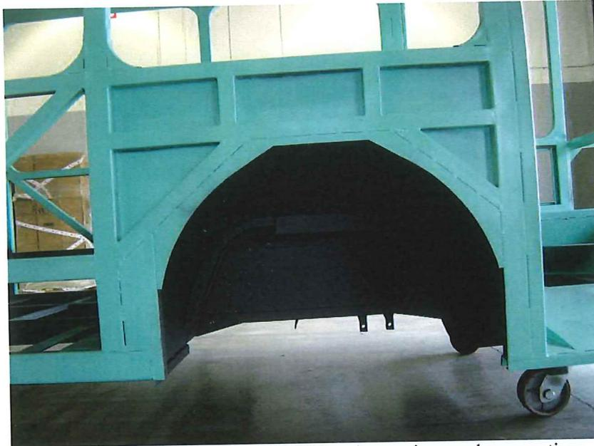
5. In critical corrosive areas, including the entire under-carriage and rear section of the bus an additional coating of PPG - Corashield #8071 is applied. The protected cage is then baked at 140°F for 20 minutes to ensure proper curing.
