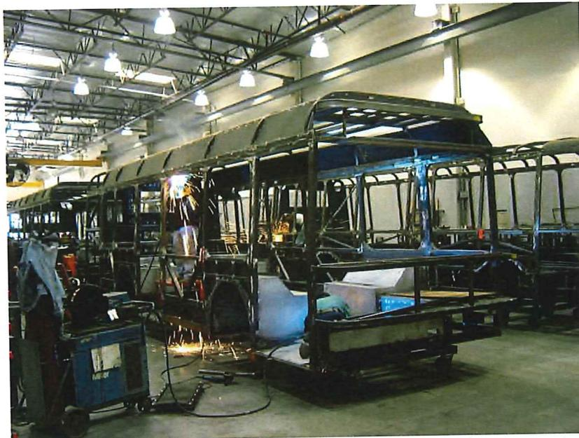
2. Completed monocoque cage construction. All welded structural components including wheelwells, stepwells and bulkheads are attached prior to the corrosion protection process.
