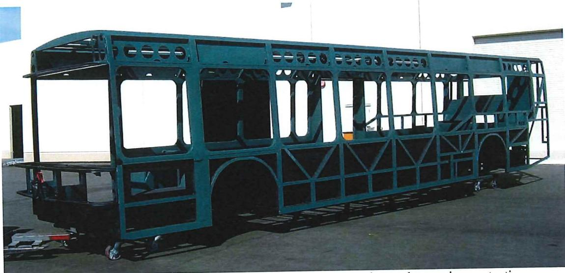
6. Low floor bus cage upon completion of the body construction and corrosion protection process. The finished corrosion protection coverage has been ASTM tested to 1,000 hours of salt spray.
