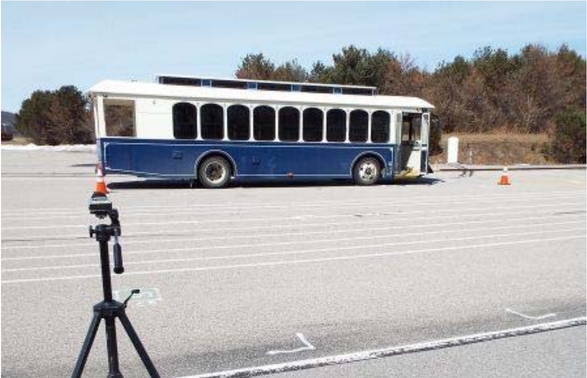
TEST BUS UNDERGOING EXTERIOR NOISE TESTING
