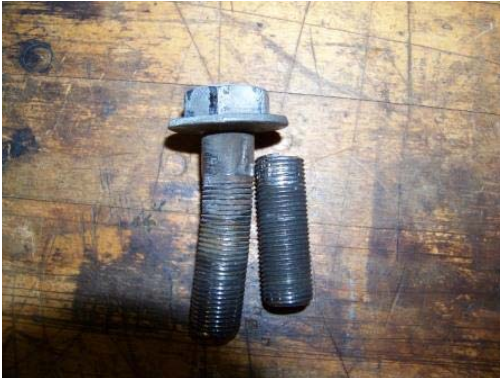
BROKEN RIGHT FRONT LOWER RADIUS ROD BOLT (1,439 TEST MILES)
