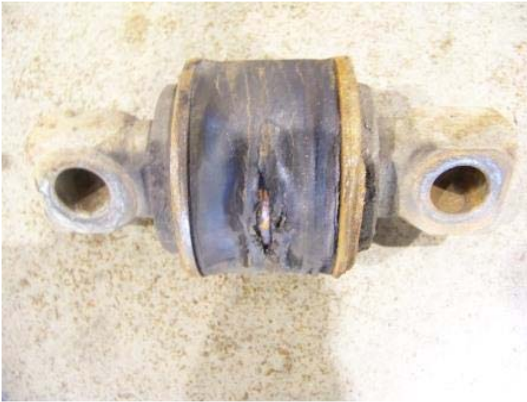
WORN FRONT LOWER RADIUS ROD BUSHING (9,008 TEST MILES)
