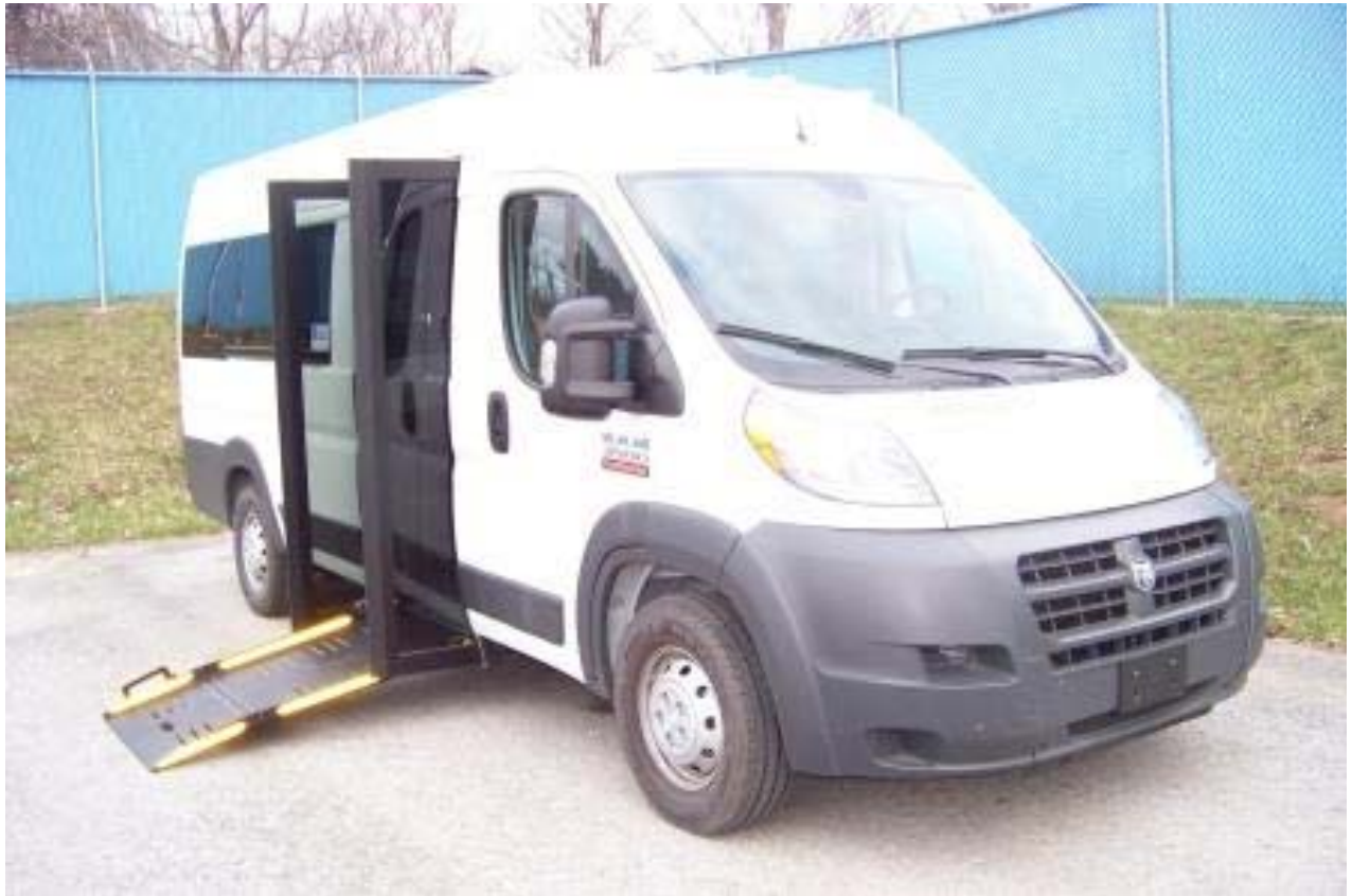
LONE STAR HANDICAP VANS, LLC. MODEL RAM PROMASTER EQUIPPED WITH A LONE STAR MODEL PMR-03 FOLD-OUT HANDICAP RAMP
