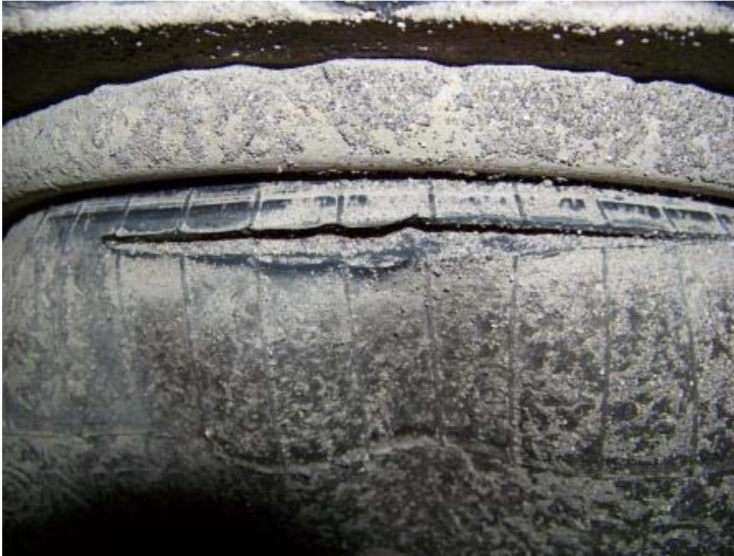
LEFT FRONT AIR BAG SEPARATING (8,760 TEST MILES)
