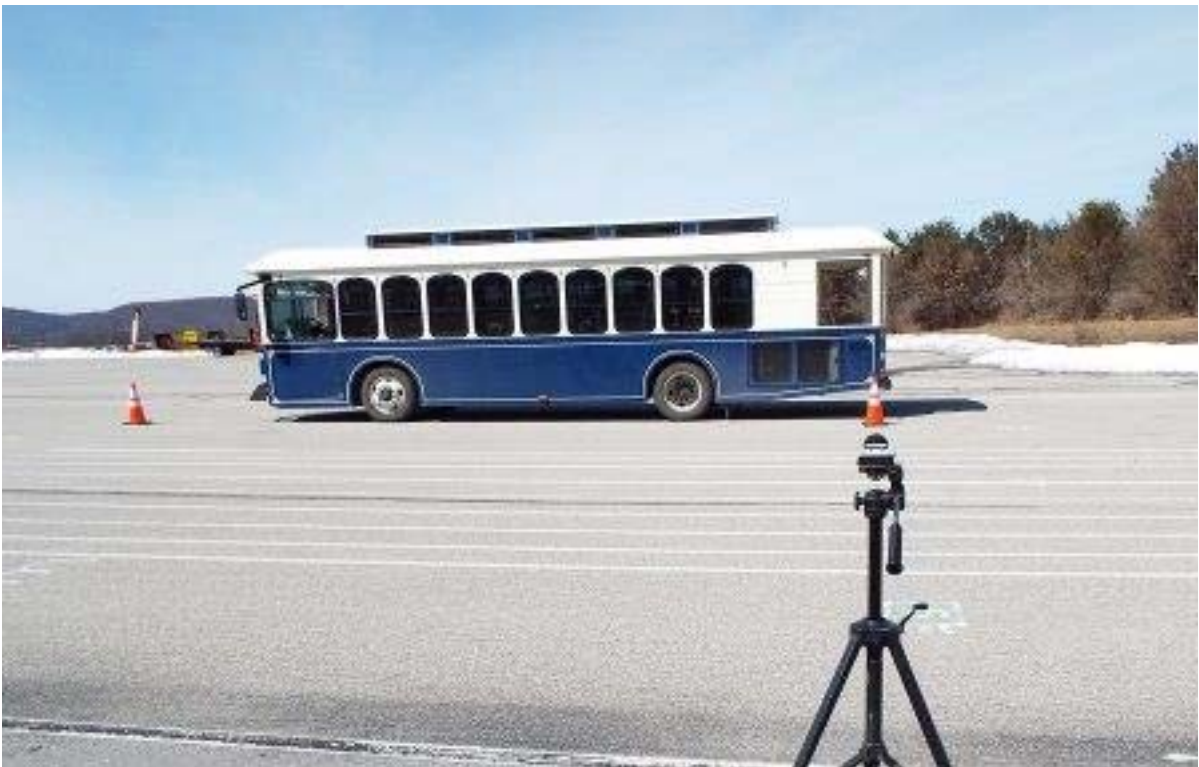
TEST BUS UNDERGOING EXTERIOR NOISE TESTING
