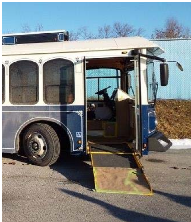
DOUBLE k Inc., dba HOMETOWN TROLLEY MODEL STREETCAR EQUIPPED WITH A BRAUN MODEL BF3262Y-2 FOLD-OUT HANDICAP RAMP
