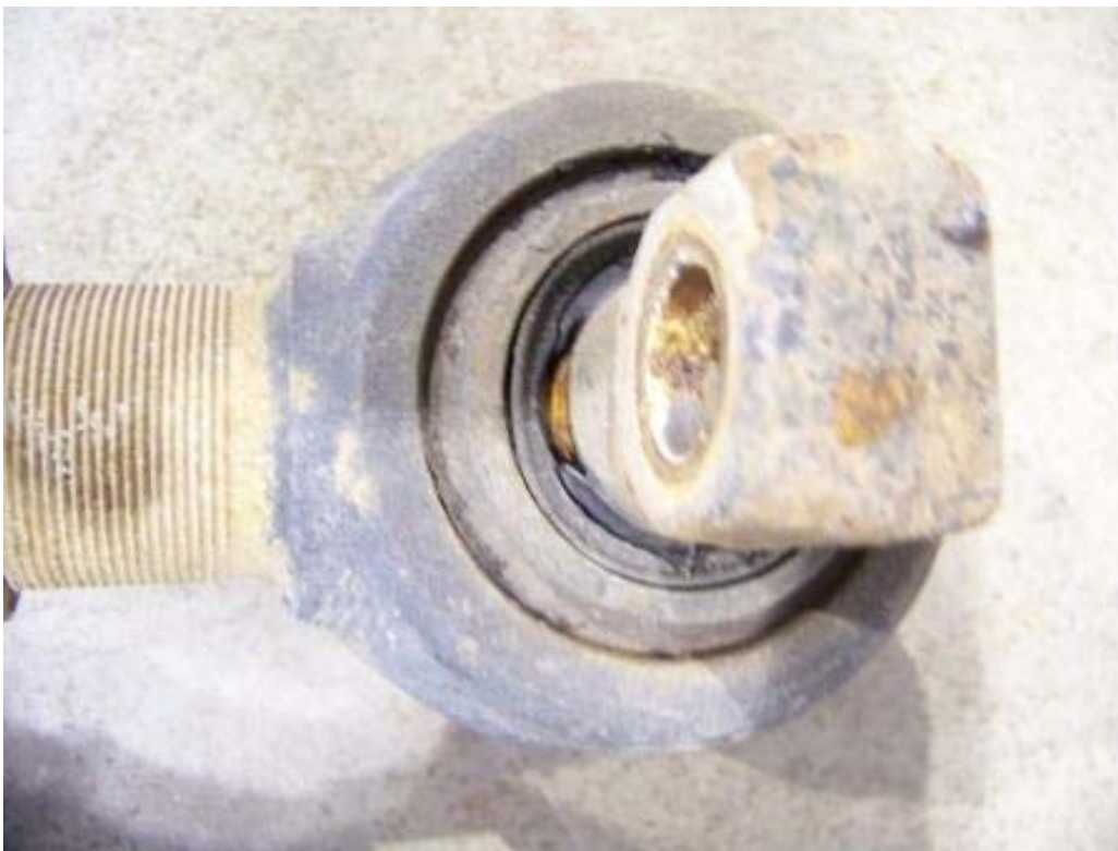
WORN FRONT LOWER RADIUS ROD BUSHING (9,008 TEST MILES)
