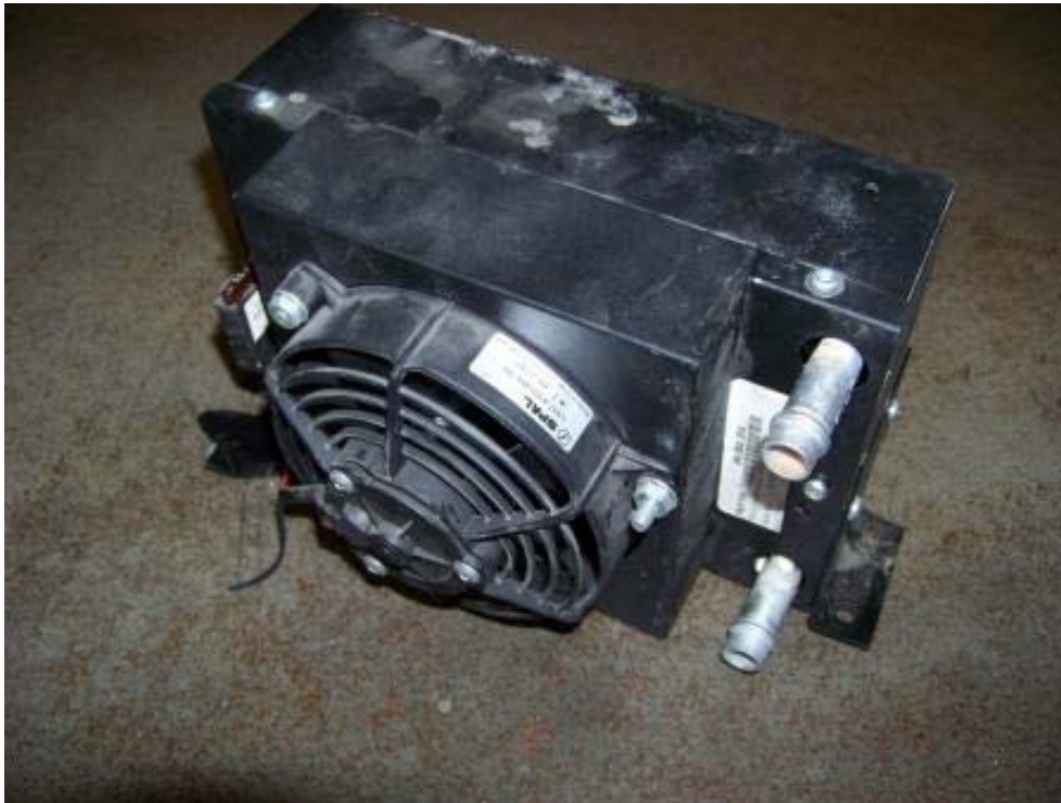
DRIVER'S HEATER LEAKING COOLANT (7,304 TEST MILES)
