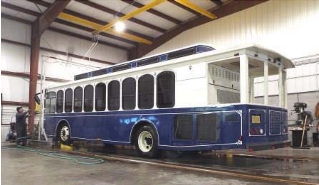
LEFT FRONT WHEEL SIX INCHES HIGHER
