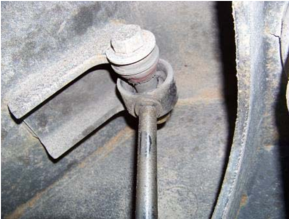
WORN LEFT FRONT UPPER SHOCK BUSHING (8,760 TEST MILES)
