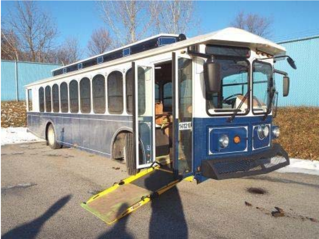
DOUBLE k Inc., dba HOMETOWN TROLLEY MODEL STREETCAR EQUIPPED WITH A BRAUN MODEL BF3262Y-2 FOLD-OUT HANDICAP RAMP
