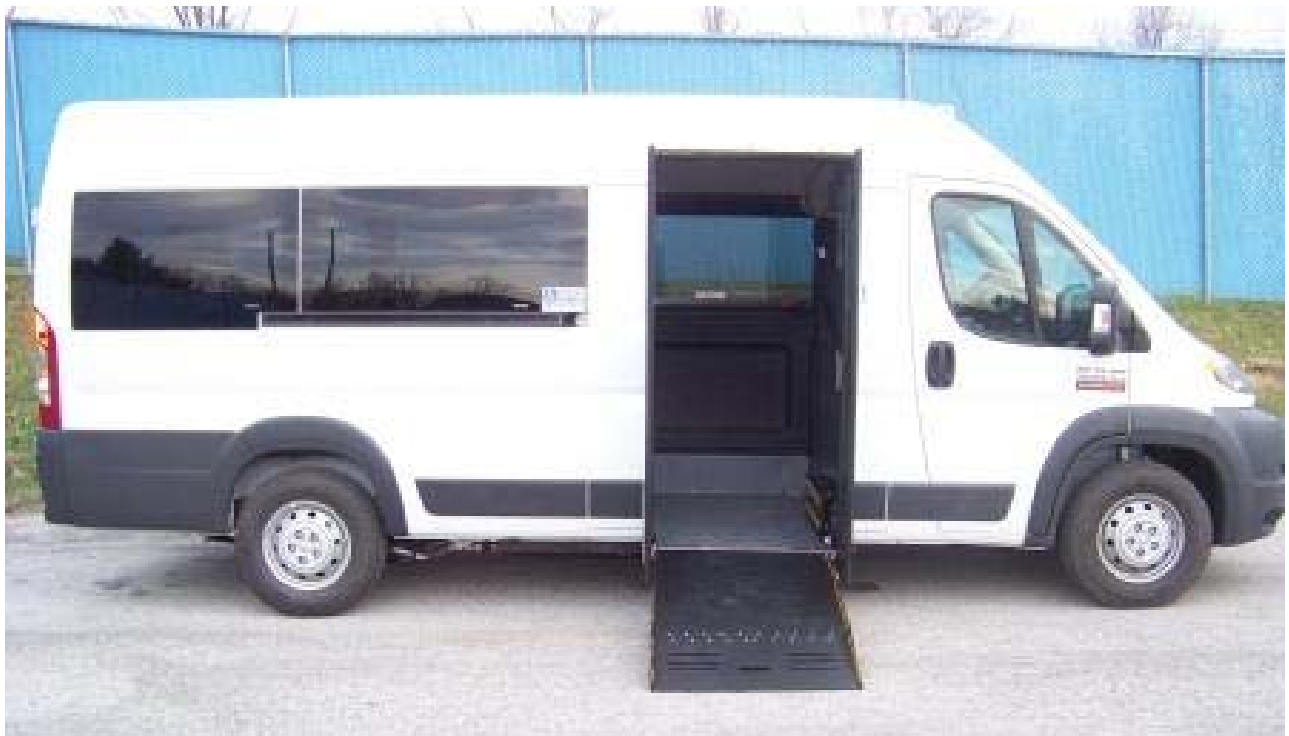
LONE STAR HANDICAP VANS, LLC. MODEL RAM PROMASTER EQUIPPED WITH A LONE STAR MODEL PMR-03 FOLD-OUT HANDICAP RAMP
