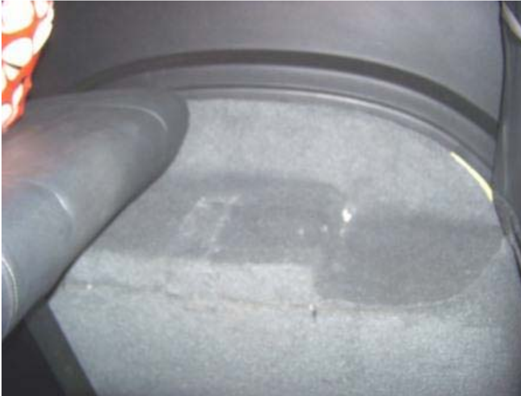
REAR WHEELS CONTACTING WHEEL WELL (215 TEST MILES)
