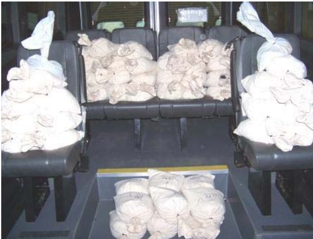
BUS LOADED TO 2.5 TIMES GVL (4,200 LBS)
