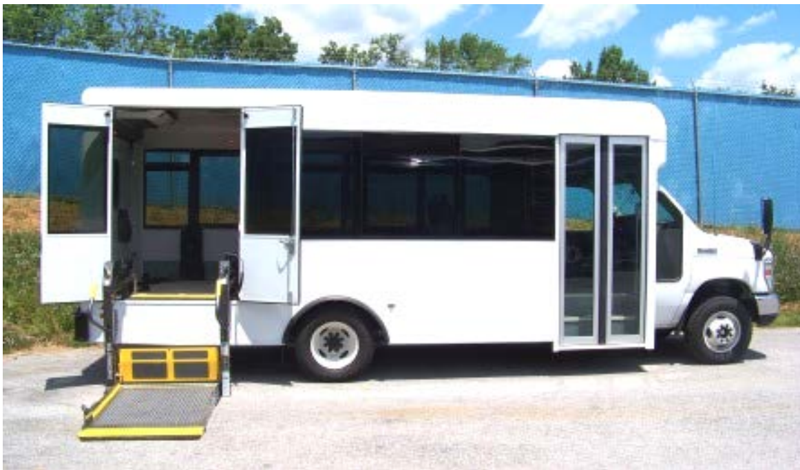
WINNEBAGO INDUSTRIES INC. MODEL E-450 EQUIPPED WITH A BRAUN CORP. MODEL N6919F1B-2 HANDICAP LIFT
