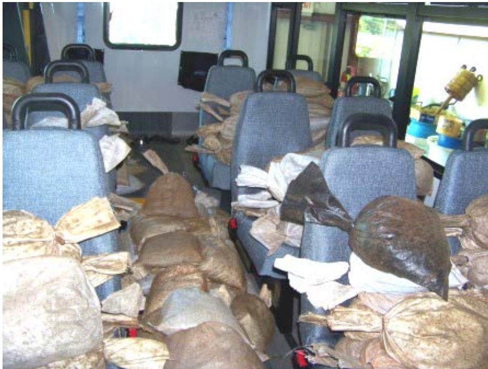
BUS LOADED TO 2.5 TIMES GVL (9,075 LBS)
