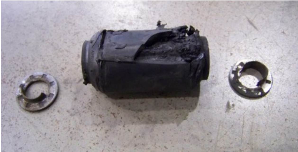
WORN SPRING HANGER BUSHINGS (4,819 TEST MILES)
