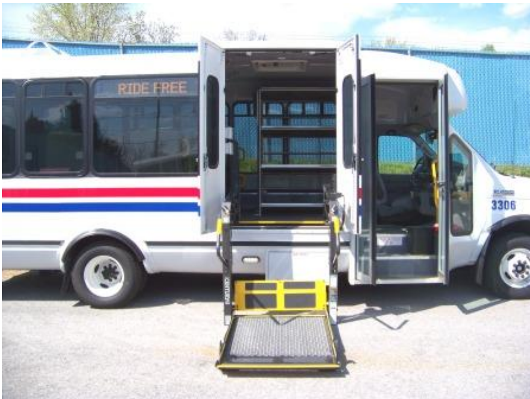
ROUSH CLEANTECH, LLC., MODEL 2011 ELDORADO EQUIPPED WITH A BRAUN MODEL NCL919FIB-2 PLATFORM LIFT
