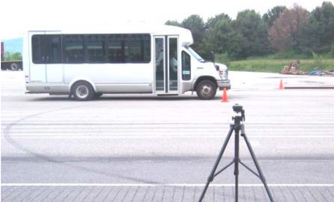
TEST BUS UNDERGOING EXTERIOR NOISE TESTING
