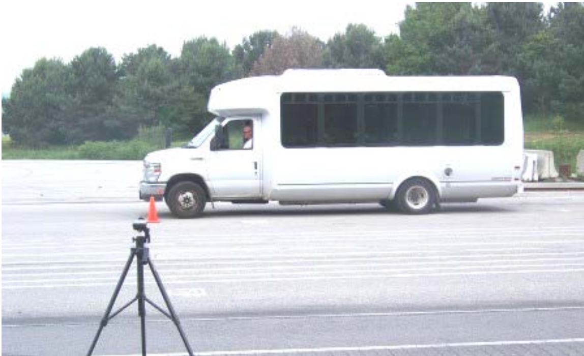
TEST BUS UNDERGOING EXTERIOR NOISE TESTING
