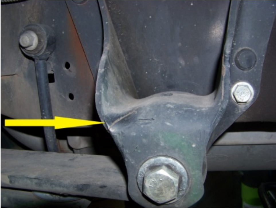
CRACKED SPRING HANGER (4,819 TEST MILES)
