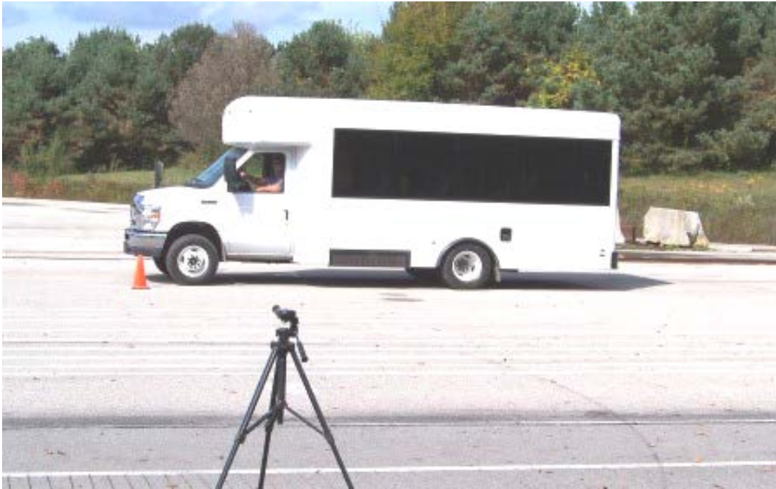
TEST BUS UNDERGOING EXTERIOR NOISE TEST
