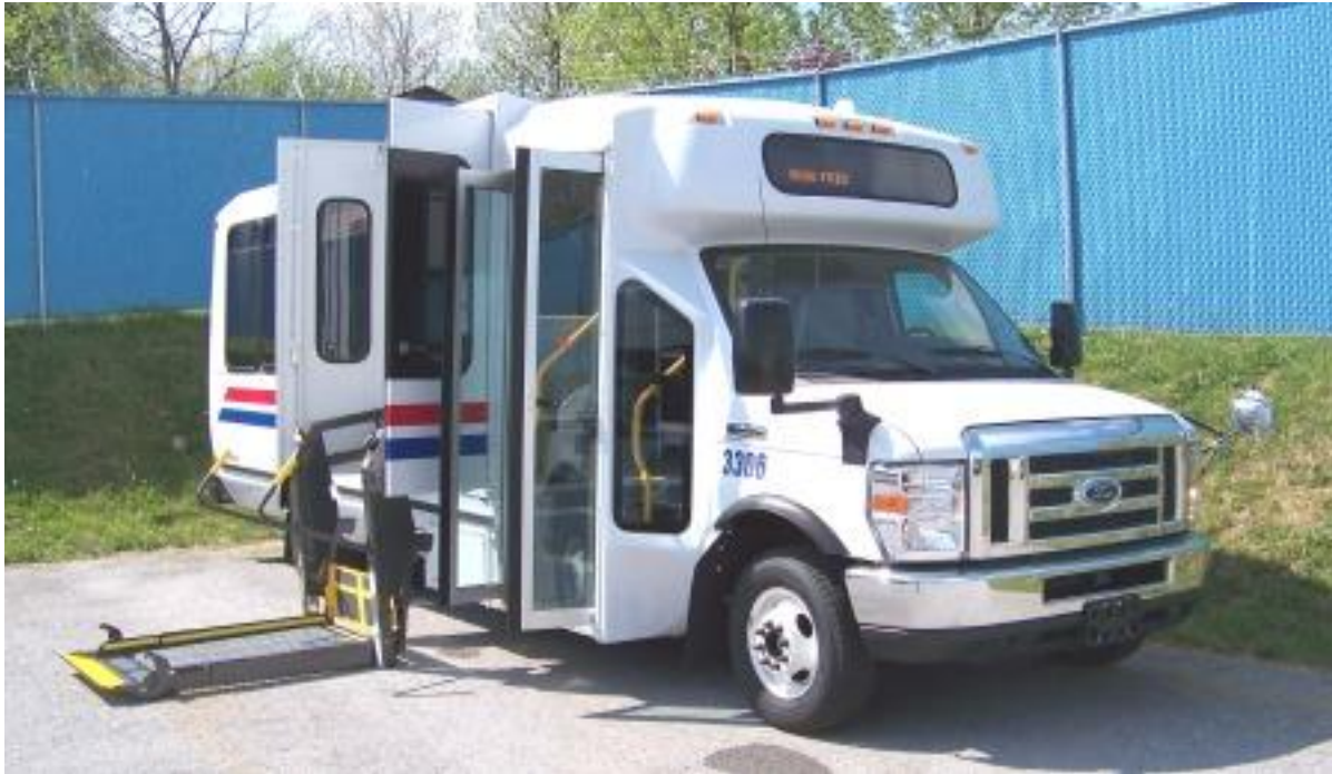
ROUSH CLEANTECH, LLC., MODEL 2011 ELDORADO EQUIPPED WITH A BRAUN MODEL NCL919FIB-2 PLATFORM LIFT
