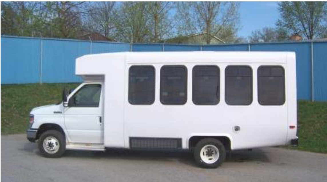
DIAMOND COACH CORP. MODEL VIP 2200 EQUIPPED WITH A BRAUN MODEL NCL919F1B-2 HYDRAULIC PLATFORM LIFT
