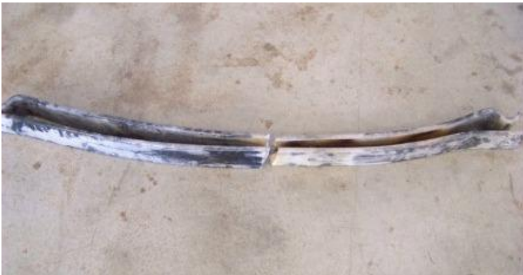
BROKEN RIGHT REAR LOAD SPRING (5,426 TEST MILES)
