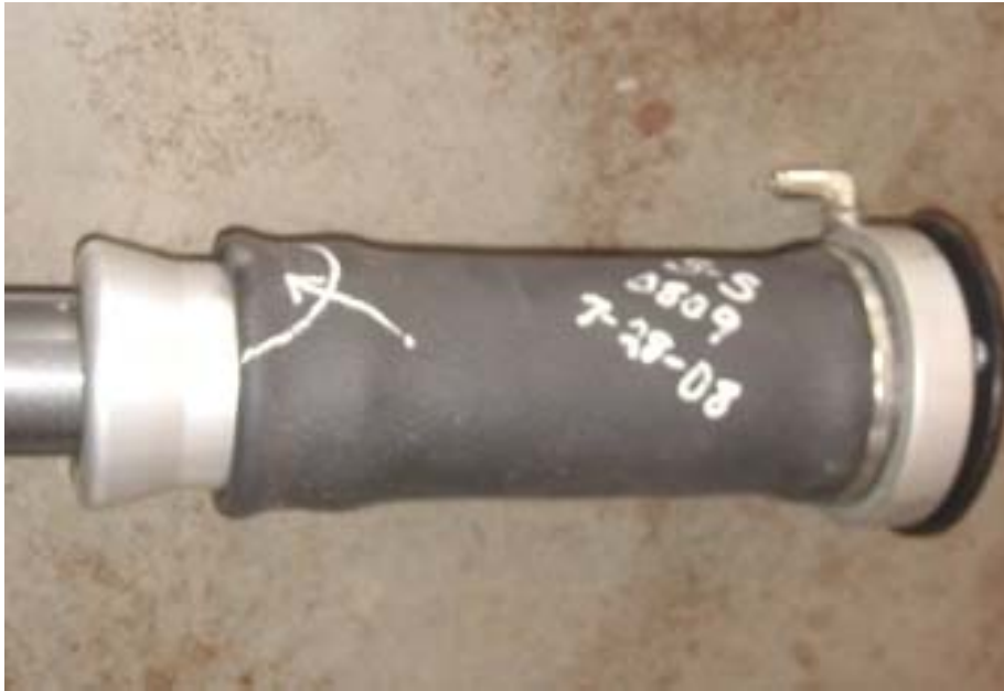
RIGHT REAR AIR STRUT IS BLISTERING (897 TEST MILES)
