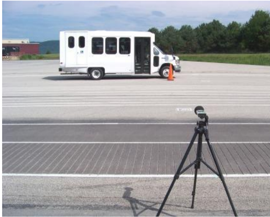
TEST BUS UNDERGOING EXTERIOR NOISE TESTING
