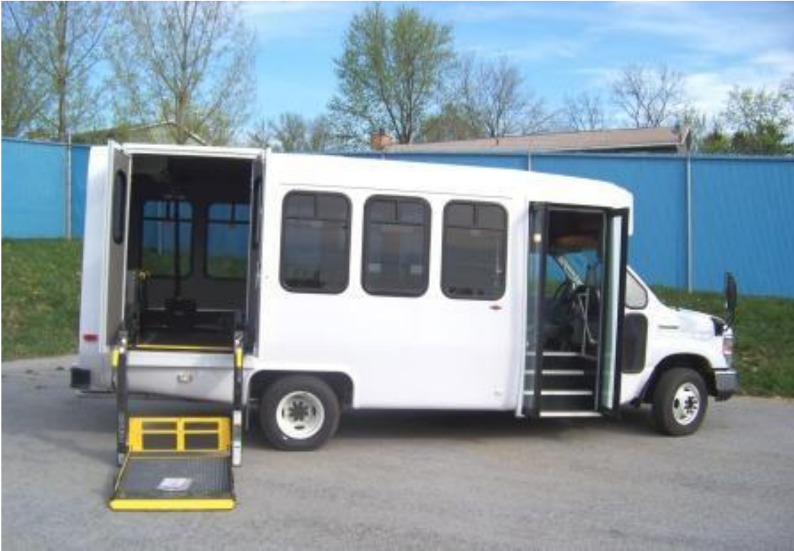
DIAMOND COACH CORP. MODEL VIP 2200 EQUIPPED WITH A BRAUN MODEL NCL919F1B-2 HYDRAULIC PLATFORM LIFT
