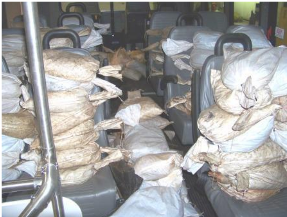
BUS LOADED TO 2.5 TIMES GVL (8,325 LBS)
