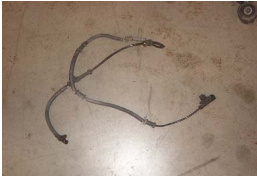
FAILED "ABS" SENSOR (2,045 TEST MILES)
