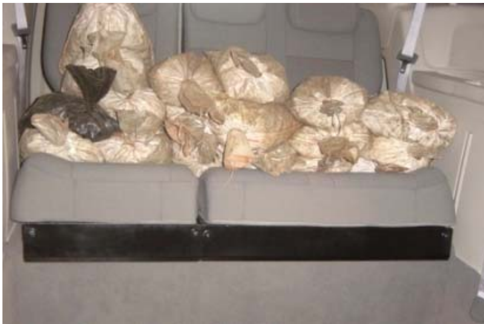
BUS LOADED TO 2.5 TIMES GVW (2,475 LBS)
