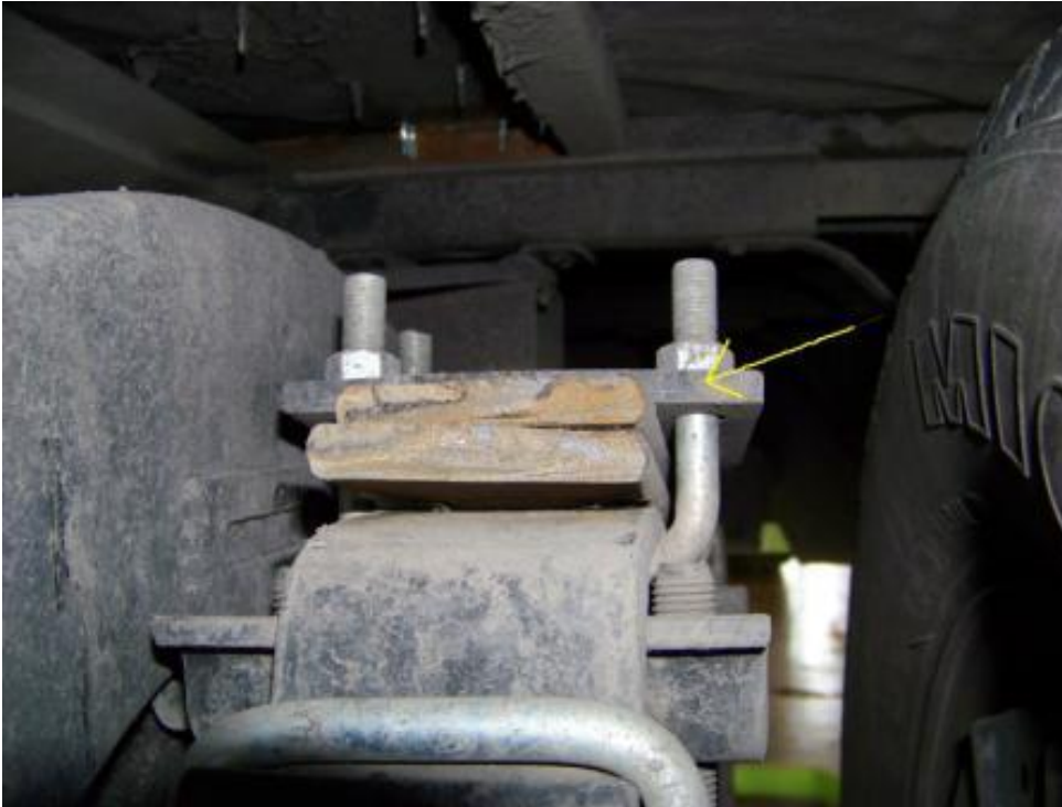
LEFT REAR SPRING: BROKEN LOWER SPRING PLY (3,073 TEST MILES)
