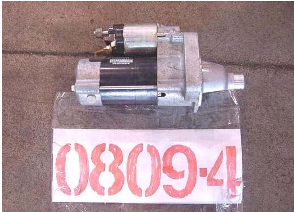
STARTER REMOVAL AND REPLACEMENT (0.75 MAN HOURS)
