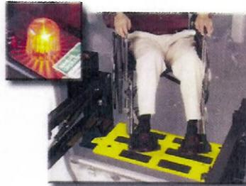
Gas spring activated outer barrier detects roll stop occupancy as the platform leaves the ground
