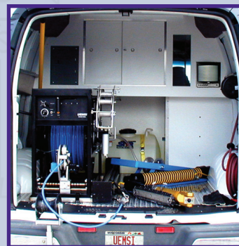
Shown above is the mainline reel, Explorer™ Zoom pan & tilt camera, and the Trax Jr.™ tractor.
