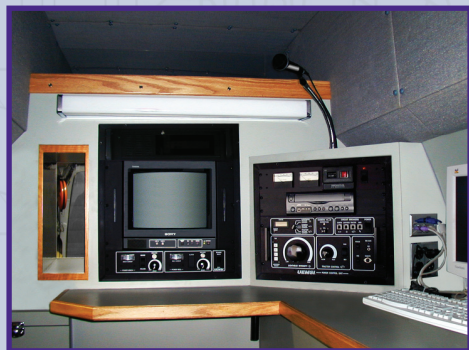
Shown above is a van control room with a Kit System engineering rack and components.
