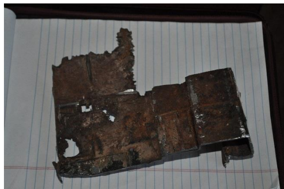
Figure 120. A portion of the corroded break metal steel sill
